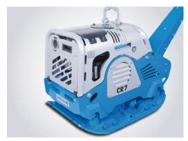
CR 7 Hd – Low overall height, powerful compaction, high-capacity gasoline engine.
