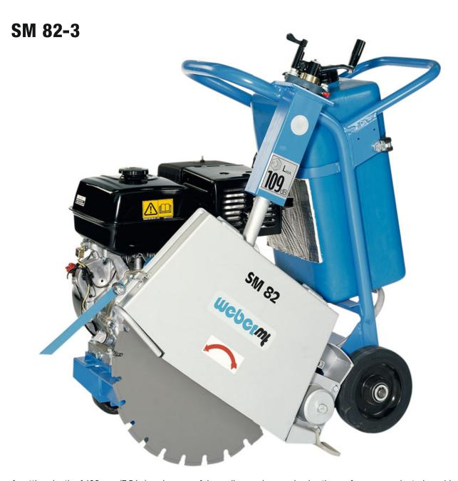
A cutting depth of 190 mm (7.5 in.) and a powerful gasoline engine emphasize the performance-oriented machine concept of the SM 82-3. Thanks to its rugged design, the machine efficiently handles a wide range of cutting tasks.
